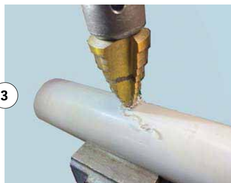
Drilling cross-arm holes in the vertical section/mast with a step drill.
