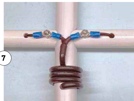
Forming the choke balun.
