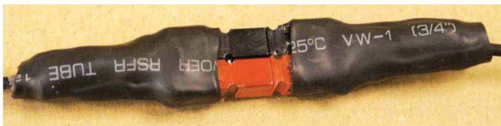
Figure 3: Powerpole connector with heat-shrink tubing filled with hot glue to give mechanical strength.
