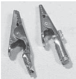
Figure 2: The alligator clip at the left has been crushed by over-tightening the thumbscrew that holds the clip securely in place. The clip at the right shows how a piece of 6-32 machine screw has been inserted into the hollow opening, preventing the thumbscrew from crushing the clip.
